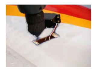
4 Use the safety clips (buy separately) to secure the servo and servo extension connected.
