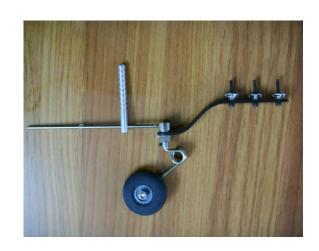
3 Use the tail wheel bracket as a template and drill holes for the mounting bolts.
