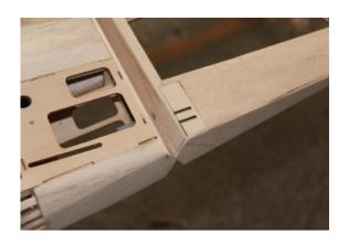
2 Fit the control horn into the slot, meansure the correct length for it
