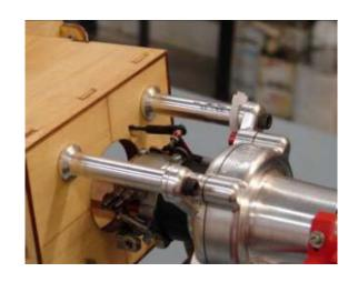
5 Insert the throttle servo into the servo mounting tray with an output arm forward.
