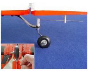
7 Epoxy the steering tube in place as shown.
