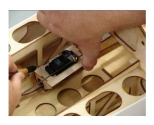
7 Use a drill to drill the servo mounting holes. Install the servo with servo screws.
