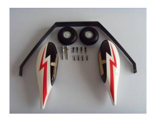
1 Install the landing gear in the pre-drilled holes with the supplied bolts and locking nuts.
