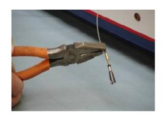
11 A drop of thin CA may be applied to the brass tube to help secure the cable
