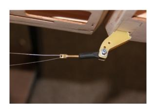
8 Drill holes for the mounting screws. Fit the servos as shown with the servo label facing the rudder. Harden the area around the holes with a drop of thin CA.
