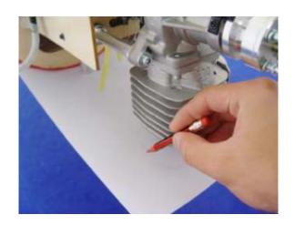
2 Use a fiber cutting tool to rough out the cowl and finish with a round sander.
