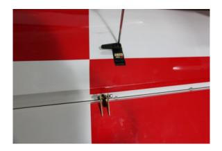
7 Install the control horn.
