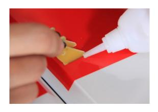
3 Drill holes for the servo mounting screws and harden the wood around the holes with a drop of thin CA.
