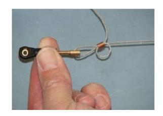
10 Crimp the brass tube with a crimping tool or pliers
