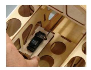
6 Mark a line for the throttle servo tray, then glue it to the fuselage.
