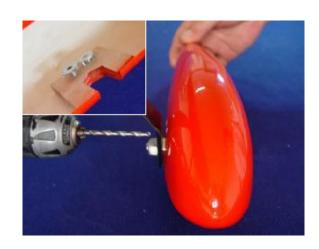
5 Drill the holes for the attached bolts and install the blind nuts as shown.
