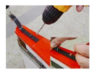
4 Install the blind nuts through the openning in the rear of the fuselage.
