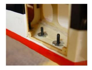
5 Install the hatch with 4 selftapping screws
