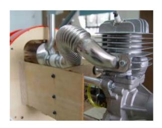
3 Use the silicone coupler and clamps to join the manifold and the canister muffler as shown.
