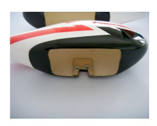
6 Mount the wheel pants and secure the bolts with a drop of Blue Loctite.
