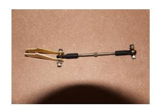
2 Put the control horn into the slot pre-opened, glue it to the stab, on each side
