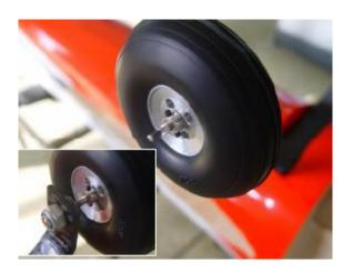
4 Slipping the wheel pant over the axles and mark the position for the two attached bolts.
