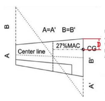
Measuer the CG from the leading edge of wing root rib. Adjust the battery pack location. For CG proper position should be at 27% MAC. This recommendation balance point is for your first flights. The CG can be moved around later to fit your personal taste.
