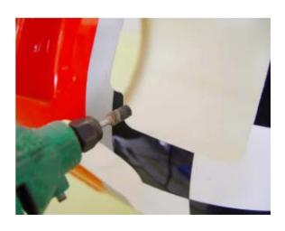
3 Use templates to cut out other opennings in the cowl for manifolds if fitted.
