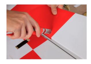
2 Fit the control horn into the slot, glue the horns into the aileron of each side.
